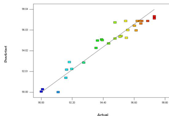
Figure 3 Plot of actual and predicted value of the conversion to biodiesel in the ultrasonic irradiation assisted biodiesel production process.
