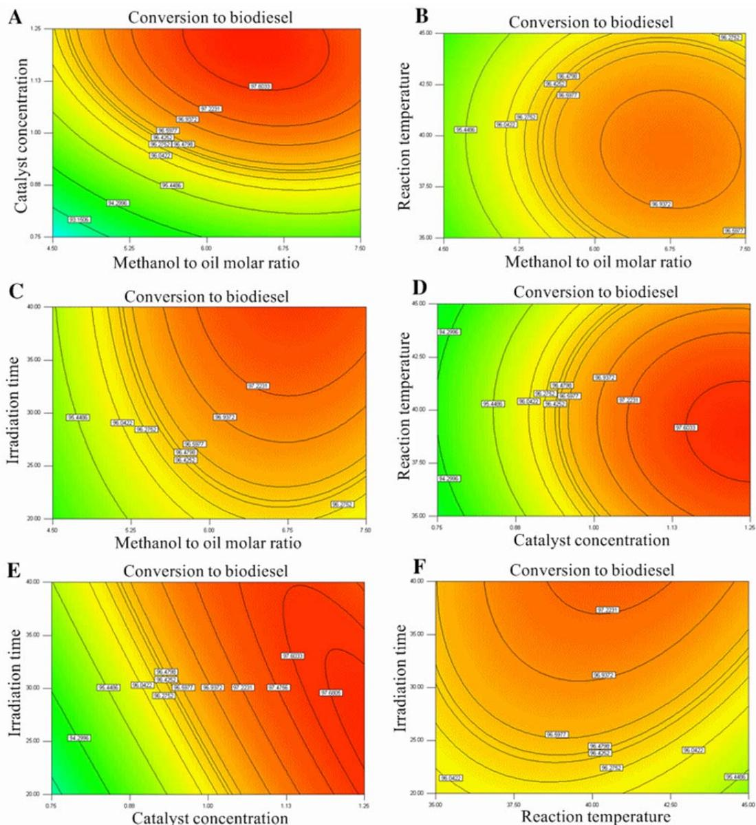
**Figure 4** Contour plot of conversion to biodiesel (wt%)
