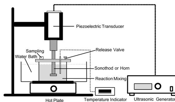
**Figure 1** Schematic representation of experiment setup used for ultrasound assisted synthesis of biodiesel from crude palm oil (CPO)
