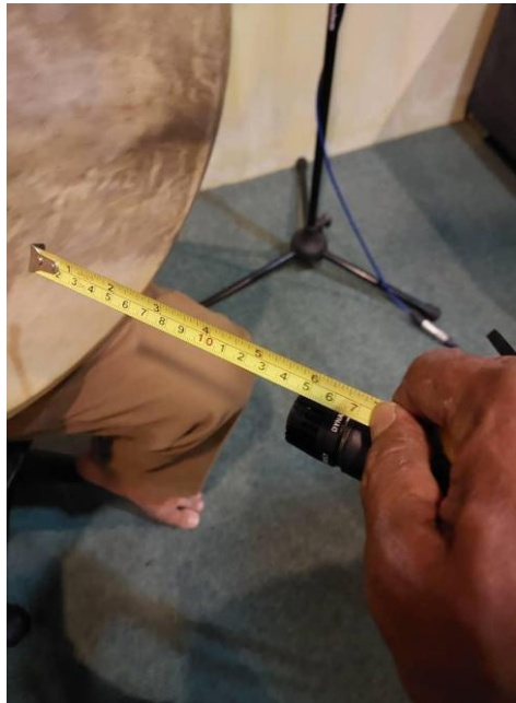
Figure 2: Microphone placed 6 inches from drumhead (Source: author).
