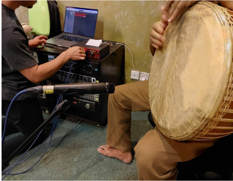
Figure 1: Microphone placed in front of rebana and recorded in Logic Pro (Source: author).
