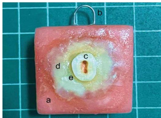
Fig. 1. Components of the experimental model: (a) cylindrical acrylic resin block, (b) metal wire loop, (c) tooth specimen, (d) freshly mixed alginate, and (e) self-cure acrylic resin.
