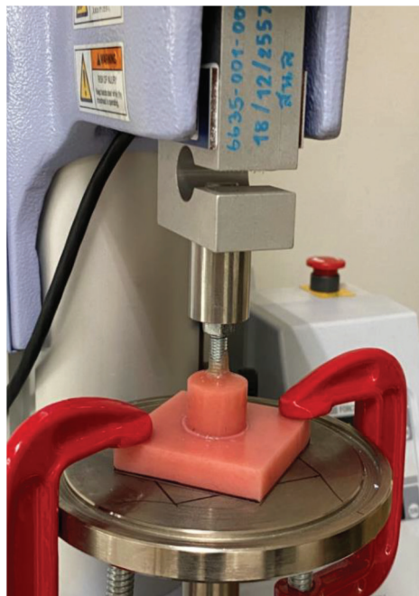
Fig 2. The sample/sample holder assembly was placed on the adhesion test instrument's sample stand, with the load applied to the sample's center up to 10.0 \pm 0.2 N at a cross-head speed of 5 mm/min.
