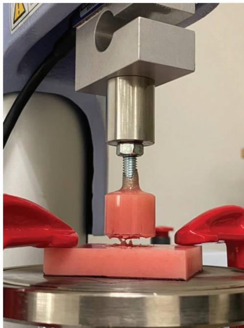
Fig 4. The pressure sensitive shaft was held with the load in place for 30 seconds, and then pulled in the opposite direction at a cross-head speed of 5 mm/min. The maximum tensile force was used for retention force testing.
