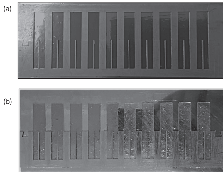
Fig 2. (a) Stainless steel mold for tear strength test specimen fabrication. (b) Tissue conditioners were packed into stainless.
