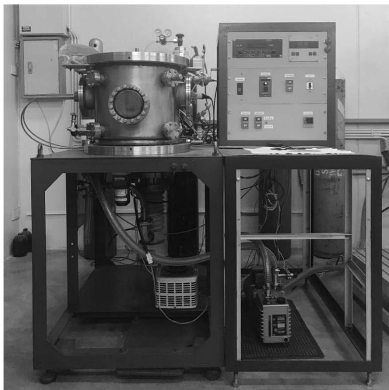
**Figure 1** Home-made DC magnetron sputtering.
