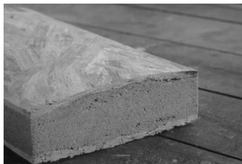
Figure 3 The prototype SIP.
