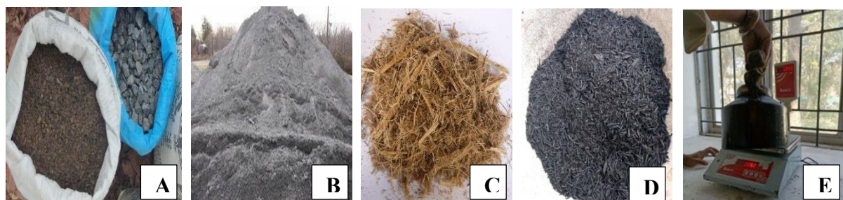
Figure 2 Raw materials for bituminous mixture preparation: A) Coarse aggregate B) Fine aggregate C) Stabilizing additive D) Raw biochar from muffle furnace E) Bitumen.
