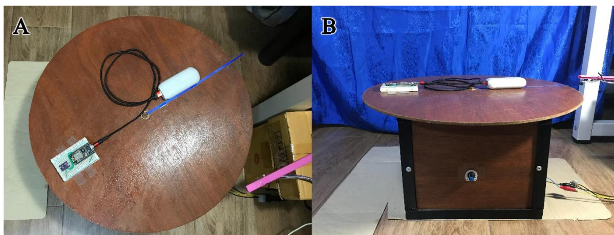
Figure 4 The sensor set was installed onto the turntable ('A' - top view and 'B' - front view).
