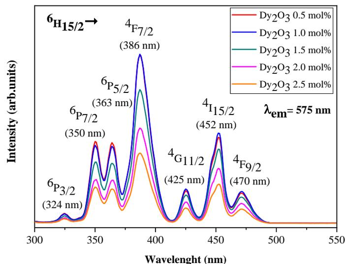
**Figure 4** The excitation spectra of the ZnO-SrO-B<sub>2</sub>O<sub>3</sub> glass at different Dy<sub>2</sub>O<sub>3</sub> concentrations.
