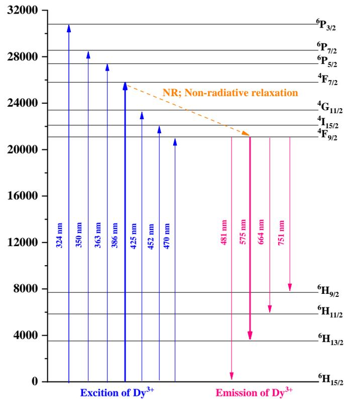
**Figure 6** The Partial energy levels diagram of the Dy<sup>3+</sup> ions in the ZnO-SrO-B<sub>2</sub>O<sub>3</sub> glass.
