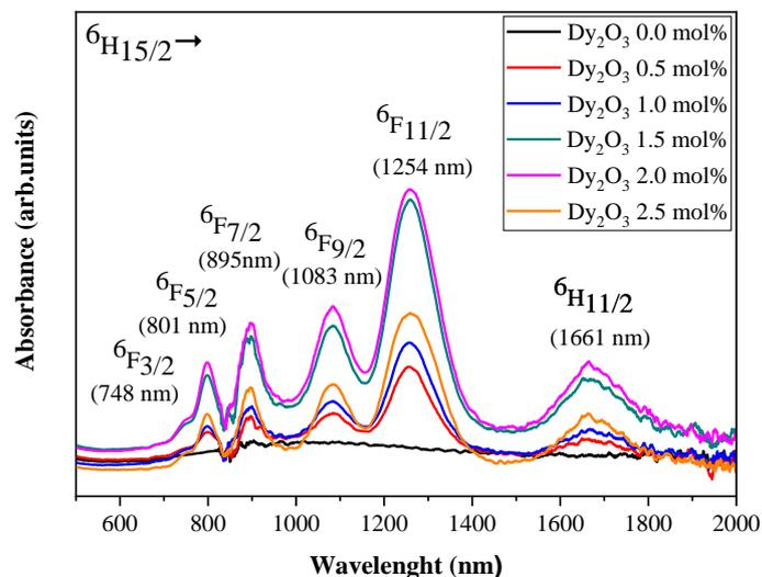
**Figure 3** The absorption spectra of the ZnO-SrO-B<sub>2</sub>O<sub>3</sub> glass at different Dy<sub>2</sub>O<sub>3</sub> contents.
