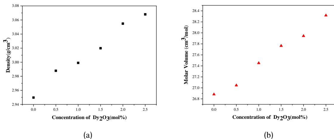
**Figure 2** (a) Variation of density ( $\rho$ ) and (b) molar volume ( $V_M$ ) for the Dy<sup>3+</sup> doped ZnO-SrO-B<sub>2</sub>O<sub>3</sub> glass.
