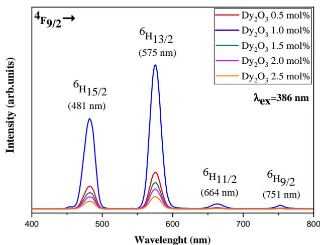
**Figure 5** The emission spectra of the ZnO-SrO-B<sub>2</sub>O<sub>3</sub> glass at different Dy<sub>2</sub>O<sub>3</sub> contents.
