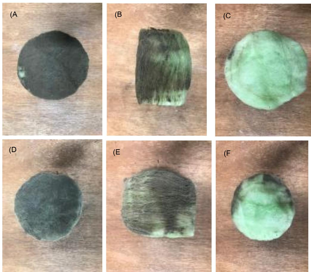
**Figure 6** Glass fiber after fume collection for regular shielding gas: front (A), side (B), and rear (C), and for nanoparticles mixed at 25 LPM and 10 grams in the canister: front (D), side (E), and rear (F).
