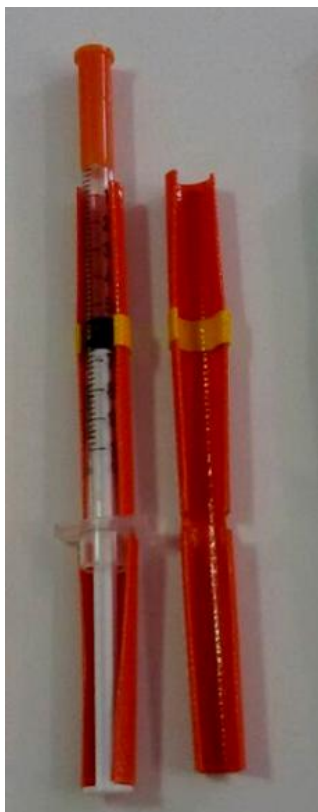
Figure 1 Prototype of the syringe drawing device to reduce dosing made of plastic straw and colored sticky paper tape.
