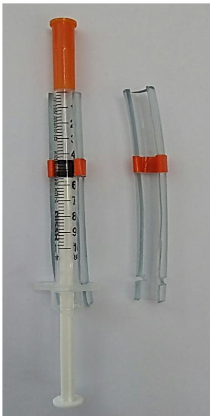
Figure 2 Improved prototype of the syringe drawing device to reduce dosing made of the clear silicone tube after the first round of satisfaction test by five healthcare providers.
