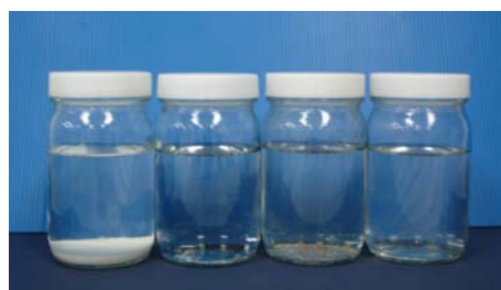
Figure 12 Appearance of systems containing propranolol HCl in IPA, 90:10 isopropyl alcohol and water, water, and 50:50 ethanol and dichloromethane, respectively (left to right).
