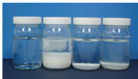
Figure 11 Appearance of systems containing lactose in water, 50:50 ethanol and dichloromethane, 90:10 isopropyl alcohol and water, and IPA, respectively (left to right).
