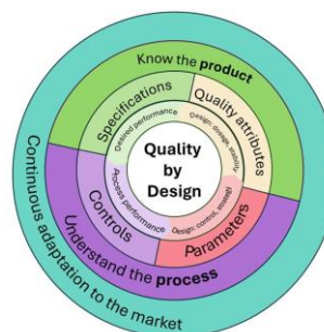
Figure 3 Illustration of FDA-suggested Quality by Design strategy for development of nanomedicines (adapted from Fornaguera et al. 60 ).
