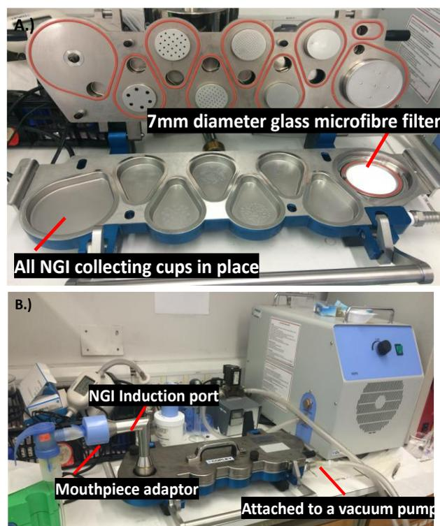
**Figure 1** Next Generation Impactor (NGI) (A) the interior structure of the NGI (B) the experimental setup.
