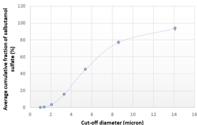
**Figure 3** Cumulative fraction of salbutamol sulfate deposited versus cut-off diameter of the respective stage of the NGI (n = 3, mean ± S.D.).
