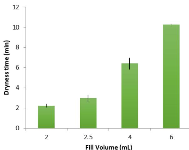
**Figure 2** Effect of fill volumes of water on time to nebulise to dryness for the vibrating-mesh nebuliser (n = 3, mean  $\pm$  S.D.).
