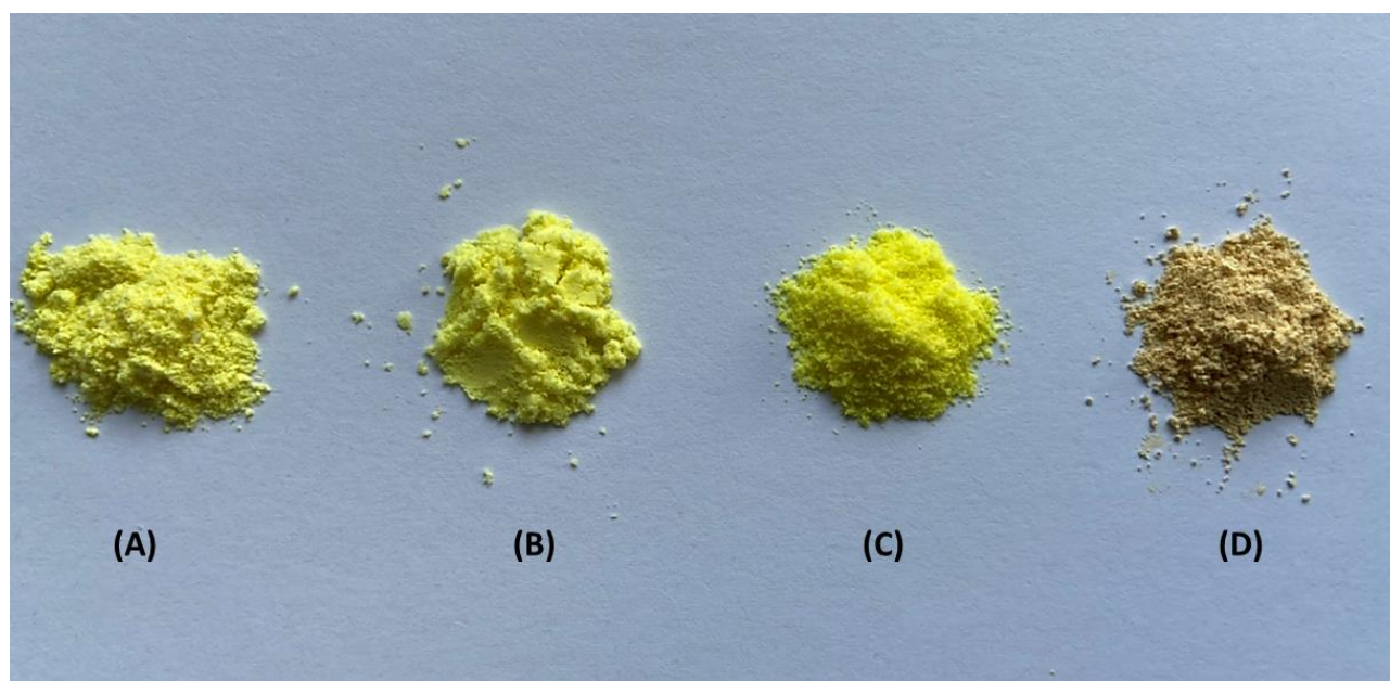
Figure 2 Solid-SEDDS of curcumin using colloidal silicon dioxide (A), lactose monohydrate (B), dibasic calcium phosphate (C) and calcium carbonate (D) as solid carriers.
