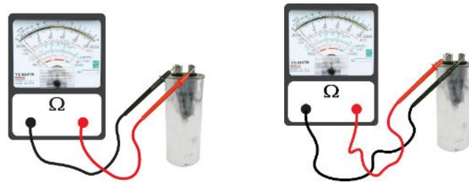
Figure 10 Verifying of the capacitor.
