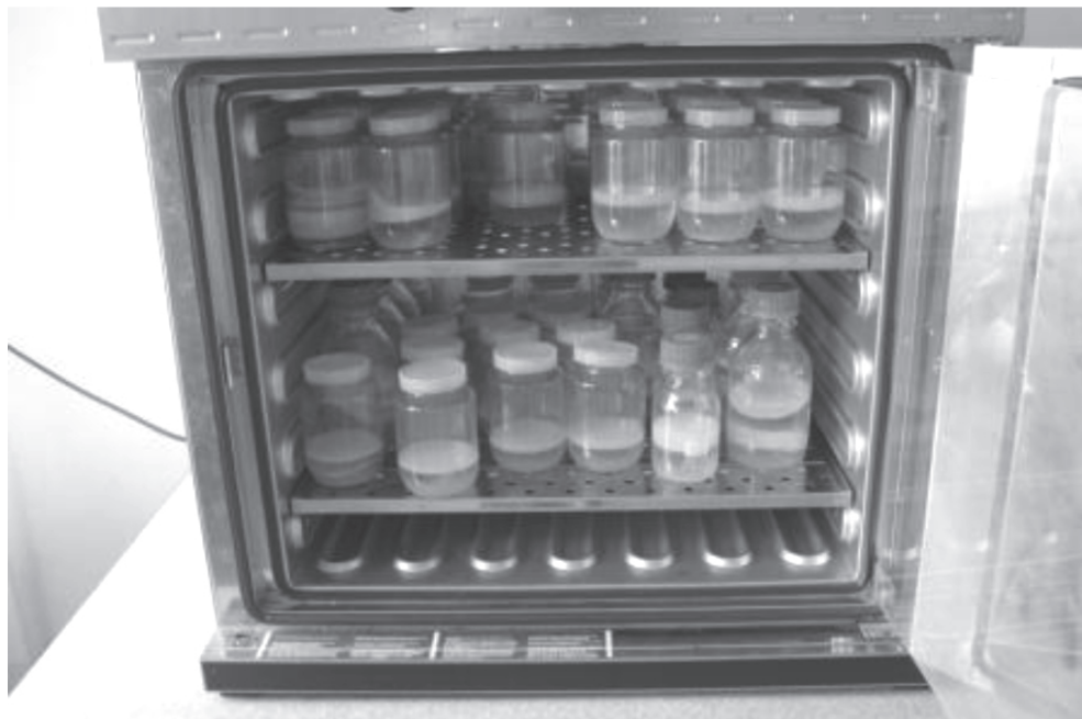
Figure 3: Maintaining the container at a constant, but not very high temperature. It is important to watch for bubbles that indicate the fermentation process is active.
