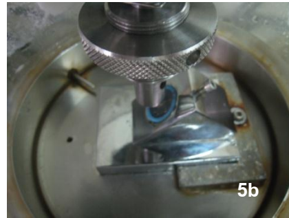
Figure 5a: The specimen restored with full metal crown mounting at 135 degree before testing in the Universal Testing Machine.
