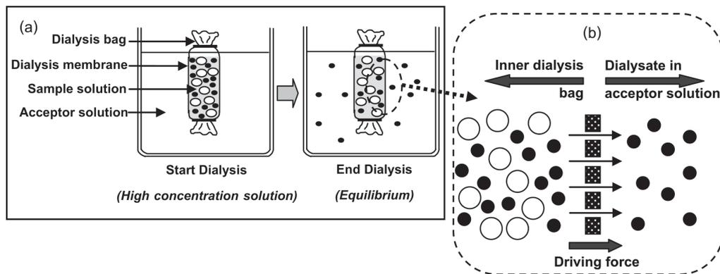
**Figure 3.** Schematic representation of (a) the conventional dialysis procedure and (b) the separation process on a dialysis membrane discriminating small solute molecules (●) and large solute molecules (○) (depicted by O. Kritsunankul and adapted from Ref. [57]).
