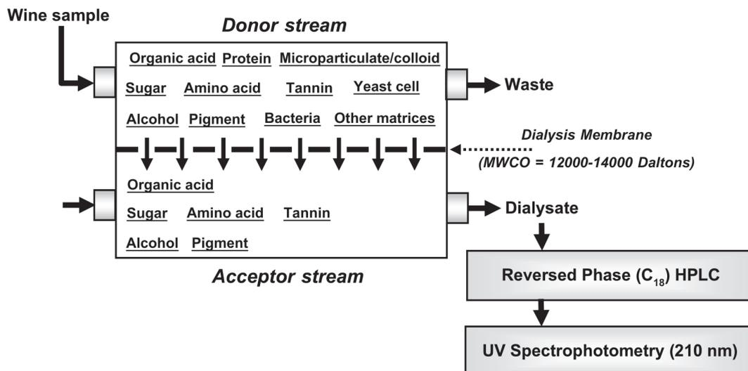
**Figure 5** Schematic representation of on-line dialysis separation process which was described by O. Kritsunankul and coworkers [11].
