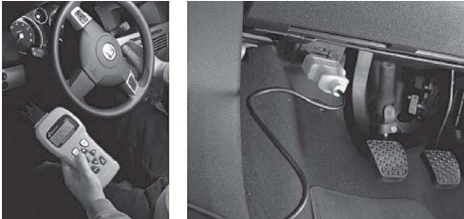
**Figure 1** An automotive scan tools into the OBD II location
