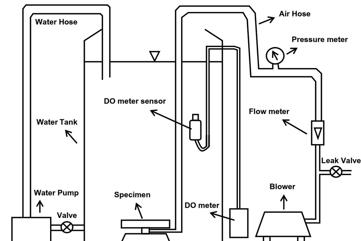
Figure 2. The schematic diagram of experiment apparatus.
