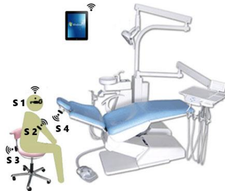
Figure 1. Intelligent ergonomic trainer composed of software Intelligent ergonomic trainer in tablet or computer running Window 8, S1 was head sensor, S2 was upper arm sensor, S3 was chair sensor, S4 was head rest sensor.
