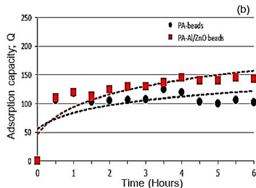
**Figure 6** The adsorption capacity of Al/ZnO NPs (a), PA-beads, and PA-Al/ZnO beads (b) for 100 mg/L synthetic melanoidins wastewater treatment
