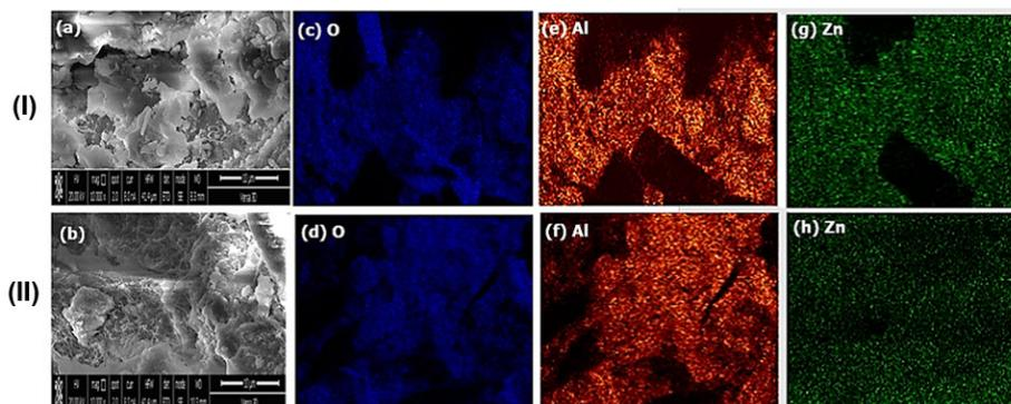
**Figure 2** Morphology and elements distribution of Al/ZnO NPs before (I) and after (II) photocatalytic decolorization of 100 mg/L synthetic melanoidins wastewater. FE-SEM (a–b) and EDX elemental distribution (c–h).
