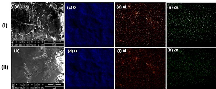
**Figure 4** Morphology and elements distribution of PA-Al/ZnO beads before (I) and after (II) photocatalytic decolorization of 100 mg/L synthetic melanoidins wastewater. FE-SEM (a–b) and EDX elemental distribution (c–h).
