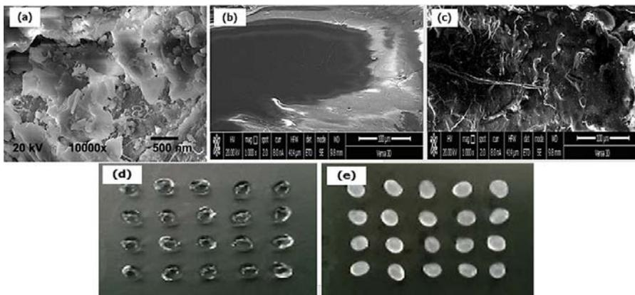
**Figure 1** FE-SEM image and morphology of Al/ZnO NPs (a), PA-beads (b and d), and PA-Al/ZnO beads (c and e).
