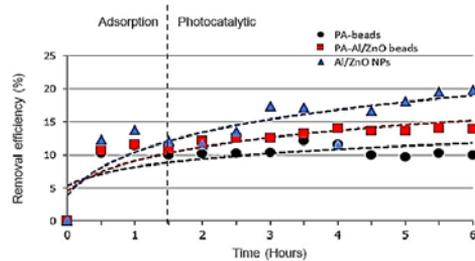
**Figure 5** The photocatalytic degradation efficiency of 100 mg/L synthetic melanoidins wastewater by Al/ZnO NPs, PA-beads and PA-Al/ZnO beads
