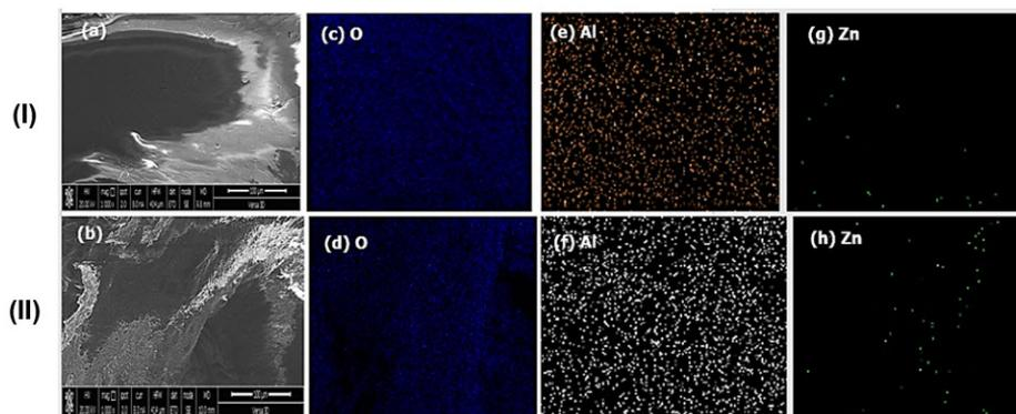
**Figure 3** Morphology and elements distribution of PA-beads before (I) and after (II) photocatalytic decolorization of 100 mg/L synthetic melanoidins wastewater. FE-SEM (a–b) and EDX elemental distribution (c–h).
