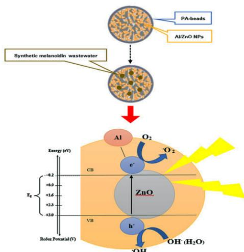
**Figure 7** Photocatalytic mechanism of PA–Al/ZnO beads for synthetic melanoidins wastewater degradation under light irradiation
